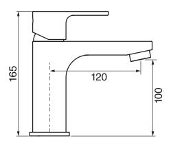
Includes push drain 3/8" flexible supply hoses 2 GPM (7.5 L/min.)
