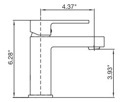
Includes push drain 3/8" flexible supply hoses 1.5 GPM (5.7 L/min.)
