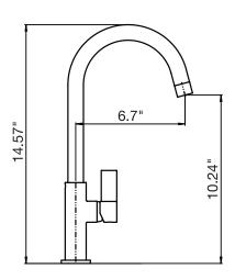
Swivel spout 1.75 GPM (6.6 L/min.)
