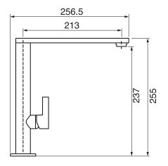
Swivel spout 1.75 GPM (6.6 L/min.)
