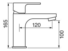
Lead free brass Includes push drain 3/8" flexible supply hoses 2 GPM (7.5 L/min.)
