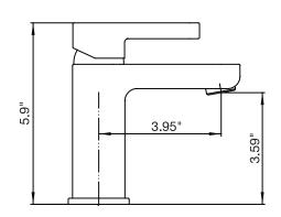
Includes push drain 3/8" flexible supply hoses 1.5 GPM (5.7 L/min.)
