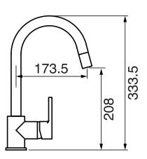
Pull down aerator Swivel spout 1.75 GPM (6.6 L/min.)
