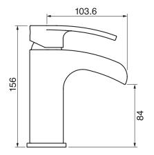
Includes push drain 3/8" flexible supply hoses 2.2 GPM (8.3 L/min.)
