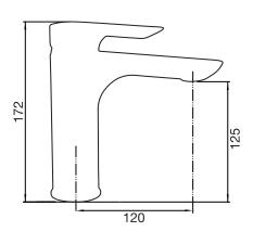
Includes push drain 3/8" flexible supply hoses 1.5 GPM (5.7 L/min.)
