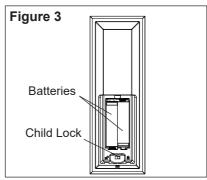
! NOTE: When the "BAT" symbol is present on the remote control it is recommended to replace the batteries promptly, to maintain full functionality of the remote/fireplace. The remote transmitter has a battery backup time of only several hours.
