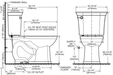
THIS COMBINATION IS DESIGNED TO ROUGH-IN AT A MINIMUM DIMENSION OF 305MM (12") FROM FINISHED WALL TO C/L OF OUTLET. \* DIMENSIONS SHOWN FOR LOCATION OF SUPPLY ARE SUGGESTED. SUPPLY NOT INCLUDED WITH FIXTURE AND MUST BE ORDERED SEPARATELY.
